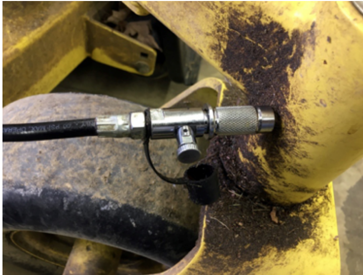
TE5699 automatic grease-fitting coupler
