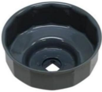
**End cap oil filter wrench:** They come in many different sizes and in some cases of a recessed oil filter, this is about all you can use. Unfortunately with a really stuck or odd shaped oil filter these are just going to spin. Also with some Fram filters that have the rubber easy to install end-coating these will not even fit. You just slip the correct size over the end of the filter and try to remember 'righty tighty – lefty loosy.'
