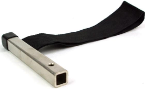
We sell a lot of [cloth strap wrenches](#) for removing large oil filters as well as unscrewing the covers off of cartridge style filters. These also do a wonderful job of removing the normal filter without damage. You just slip the strap and turn until the slack is out. Then you can use a ratchet wrench or breaker bar to turn the filter/cover loose.
